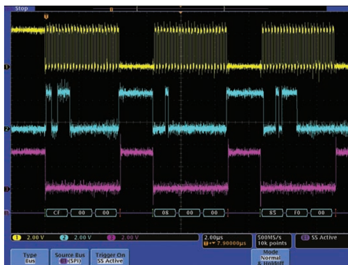
Figure 12. Acquiring synthesizer configuration messages off the SPI bus.
