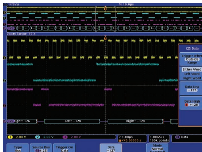
Figure 48. Triggering outside a range of values on an I 2 S bus.
