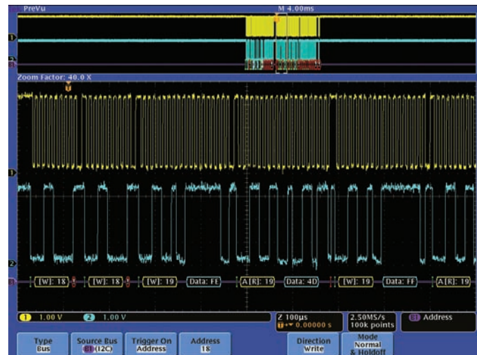
Figure 7. I 2 C address and data bus waveform decoding.
