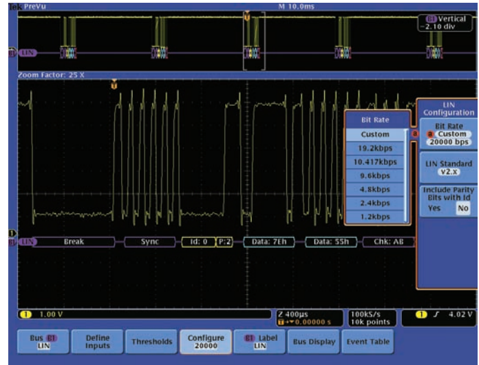
Figure 34. LIN bus setup menu and decoded frame.
