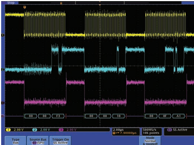
Figure 13. Correct synthesizer configuration messages.
