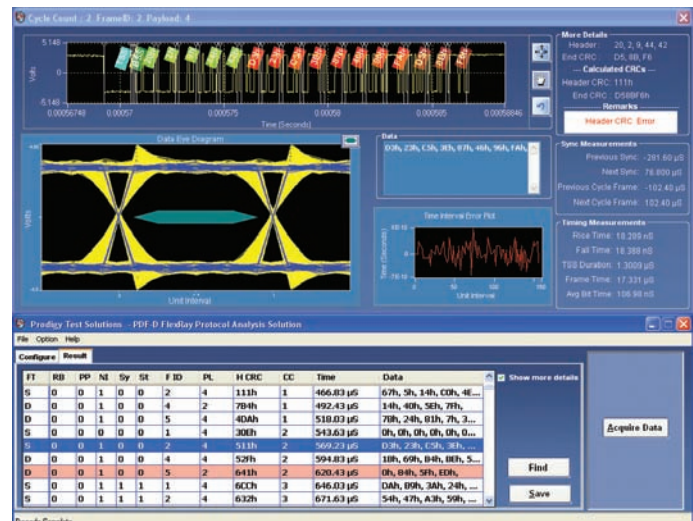
Figure 43. Eye Diagram analysis of a FlexRay signal.
